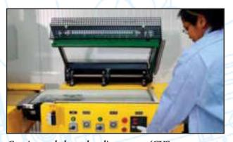
Continuously heated sealing system (CVS The continuously heated weld bar permits a high production capacity to be achieved.
