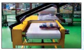
**Automatic conveyor system**Both the height and the speed of the automatic conveyor system are smoothly adjustable.
