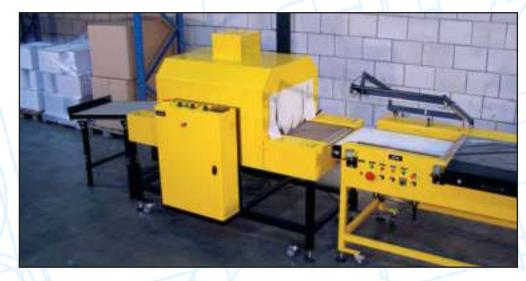
processing speed of the conveyor rollers is smoothly adjustable. The easily readable temperature is controlled and maintained electronically. Another great advantage is that all AVC shrink tunnels are equipped with castors as a standard feature so that they can be used in any location. The specified models are series-produced, but they can be supplemented with specific options in order to achieve the very best packaging solution.
